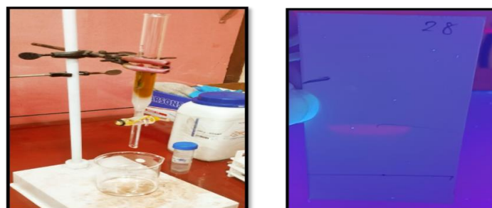
Figure 9: Silica gel column chromatography of the methanolic extract of Moringa oleifera and TLC analysis of the collected fractions.
